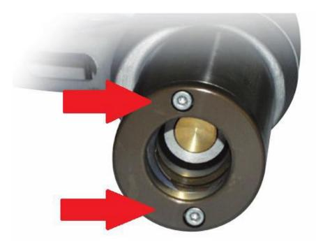
IF NOZZLE BECOMES DIFFICULT TO CONNECT OR DISCONNECT FROM VEHICLE'S FILL PORT, LUBRICATION AND THIS SCREW TORQUE CHECK IS THE FIRST COURSE OF ACTION.
